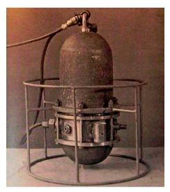
Fig. 9. The first electronic CTD probe for the *in-situ* observation of vertical temperature and salinity profiles in the upper ocean (Plate 24 in Hinkelmann, 1956). In the protective cage the one-conductor cable with oil filled connector, the pressure inlet, an electrode conductivity cell, and the platinum thermometer are shown from left to right. The upper housing was packed with dozens of thermionic valves.
