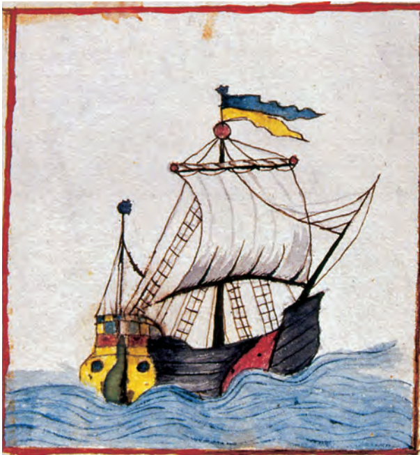
Fig. 24 A bojort depicted as the prototype for the seal of the town of Bro/Kristinehamn in Lake Vänern in 1642. In contrast to most boejer -type ships it carries a square mainsail and is probably thought of as clinker-built, in the manner of local adaptation. But the prestige of a Dutch boejer still lingers in the choice of seal. (Photo: Kurt Eriksson, Riksarkivet, Stockholm)
