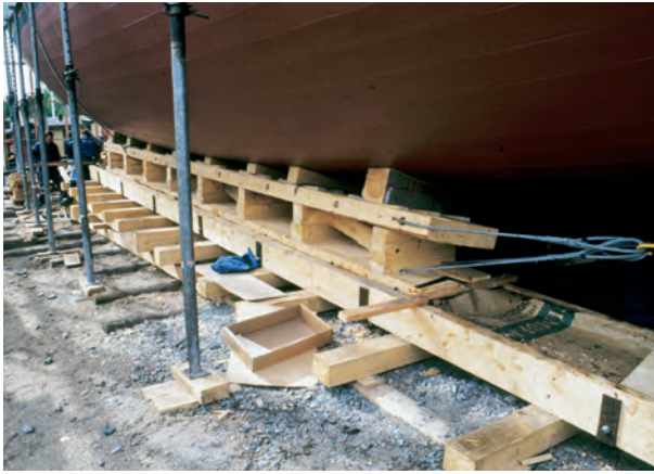
Fig. 55 The wooden tracks and sledges of a reconstruction of Jakobstads Wapen , launched in 1994 in Jakobstad. A ketch ( galeas ) with this name dating from 1767 was the first to be built and sail from the town after the partial abolishment of the Bothnian Trade Compulsion. The design was that of F.H. Chapman.
