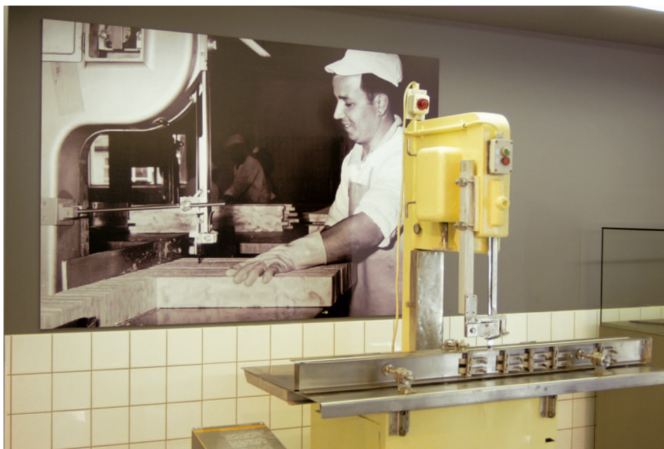
Fig. 6 An original manually operated band-saw from the early days of fish finger production. (Photo: Egbert Laska, German Maritime Museum)
