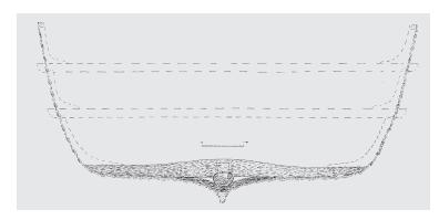
Fig. 3 Rough sketch reconstruction of the cross section of the Big Ship at the mast. (Drawing: A.E. Christensen)
